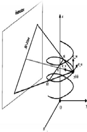
**Figure 1.** The geometry of spiral cone beam CT
