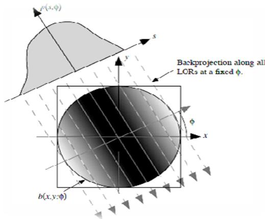
Fig 1. Back projection  $b(x,y,\emptyset)$ , into an image reconstruction array of all values  $P(S,\emptyset)$  for a fixed value of  $\emptyset$
